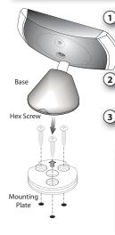
Align mounting plate to location and attach with three screws. Make sure the arrow points toward the front of the car.
