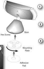
Insert mounting plate into display base and tighten hex set screw.
